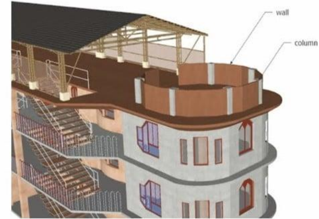
2. Addition of wall for the support
